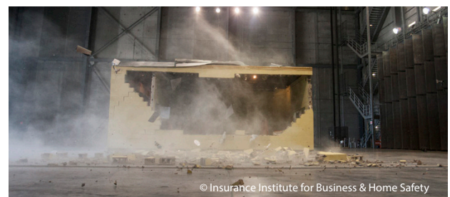
A commercial high wind demonstration at the IBHS Research Center shows the importance of using the right products and installation methods.
